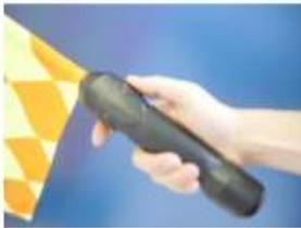
The radio transmitters are integrated in the handles of the assistant flags and send a data telegram to the receiver on the referee's arm when the button is pressed. As a control, a pulsating, even vibration can be felt on the handle. The flagpole is screwed into the handle and can be easily replaced. The battery cover (with bayonet lock) can also be removed or attached by turning it slightly
